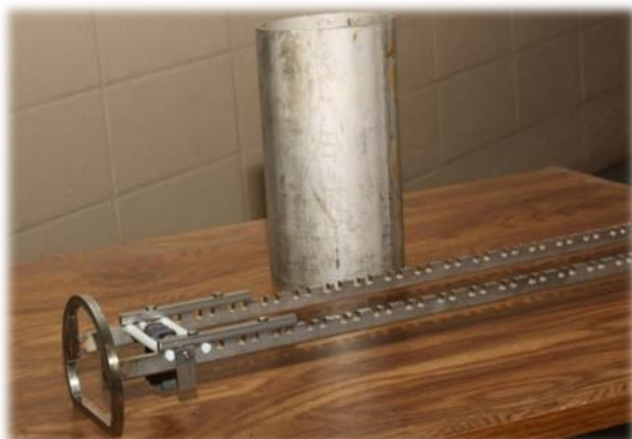
In-pipe Corrosion Coupon Racks
